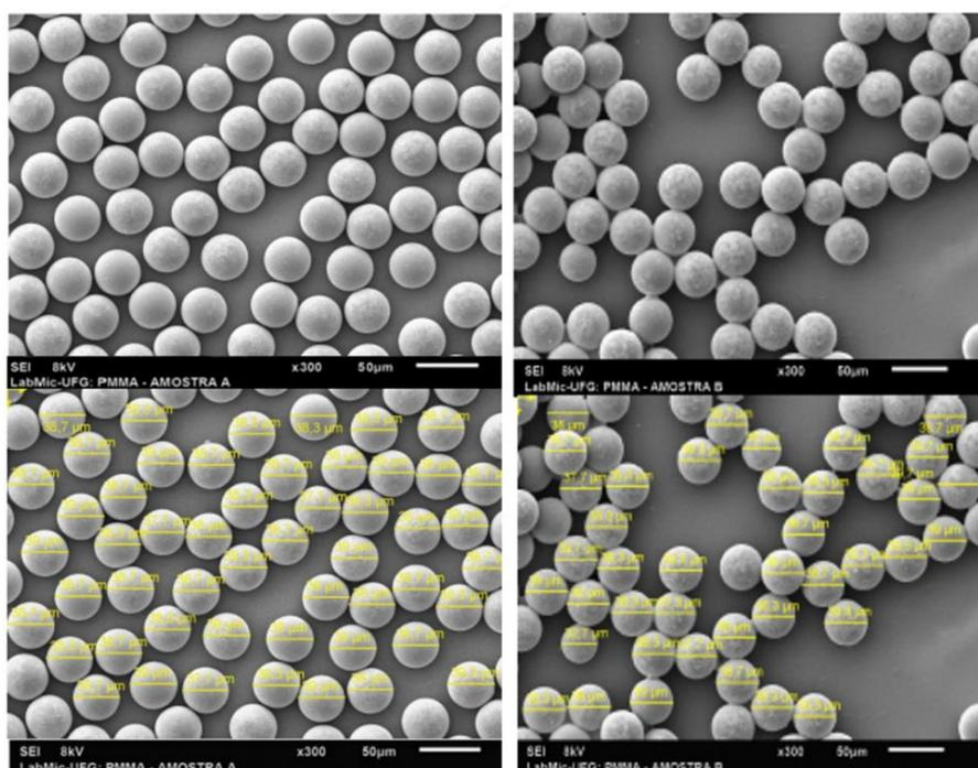
In this study, 1,531 (one thousand five hundred and thirty-one) particles were measured in sample A and 1,522 (one thousand five hundred and twenty-two) in sample B. The result is shown in the size distribution in **Figure 2**.
